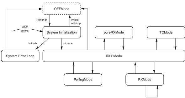
After connecting the supply voltage to the VS pin, the Atmel ATA5781/2/3 always starts in OFFMode. All internal circuits are disconnected from the power supply. Therefore, no SPI communication is supported. The Atmel ATA5781/2/3 can be woken up by activating the PWRON pin or one of the NPWRONx pins. This triggers the power-on sequence. After the system initialization the Atmel ATA5781/2/3 reaches the IDLEMode.
