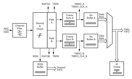
The channel filter determines the receiver bandwidth. Its output is used for both receiving paths A and B, making it necessary to configure the filter to match both paths. The receiving paths A and B are identical and consist of an ASK/FSK demodulator with attached signal checks, a frame synchronizer which supports pattern-based searches for the telegram start and a 1-byte hardware buffer with integrated CRC checker for the received data.
