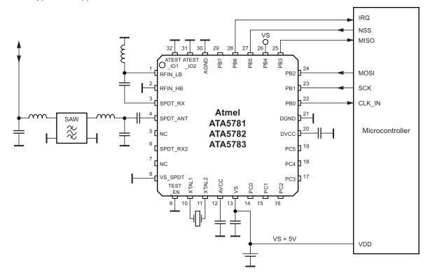
Figure 1-3 shows a typical vehicle side application circuit with an external host microcontroller running from a 5V voltage regulator. The pin PB4 (PWRON) is directly connected to VS and the Atmel ATA5781/2/3 enters the IDLEMode after power-on. In this configuration the Atmel ATA5781/2/3 can work autonomously and the  $\mu$ C stays powered down to keep current consumption low while remaining sensitive to RF telegrams.
