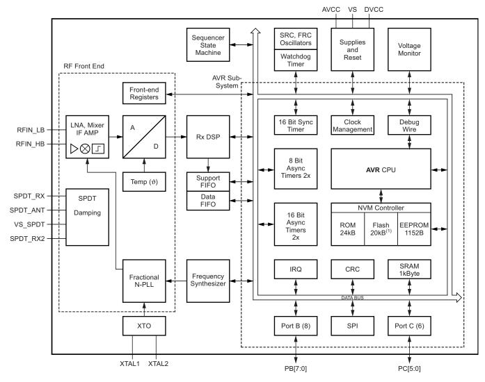
(1) 20kByte Flash for Atmel ATA5782, 20kByte user ROM for Atmel ATA5783, no user memory for Atmel ATA5781
